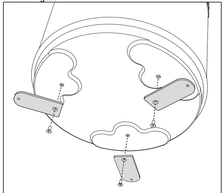
fig. 50- Fixing the brackets
