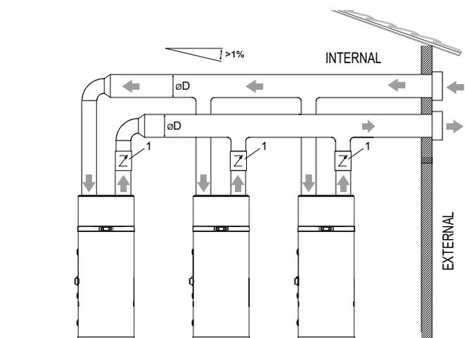
fig. 56- Example of air outlet connection
