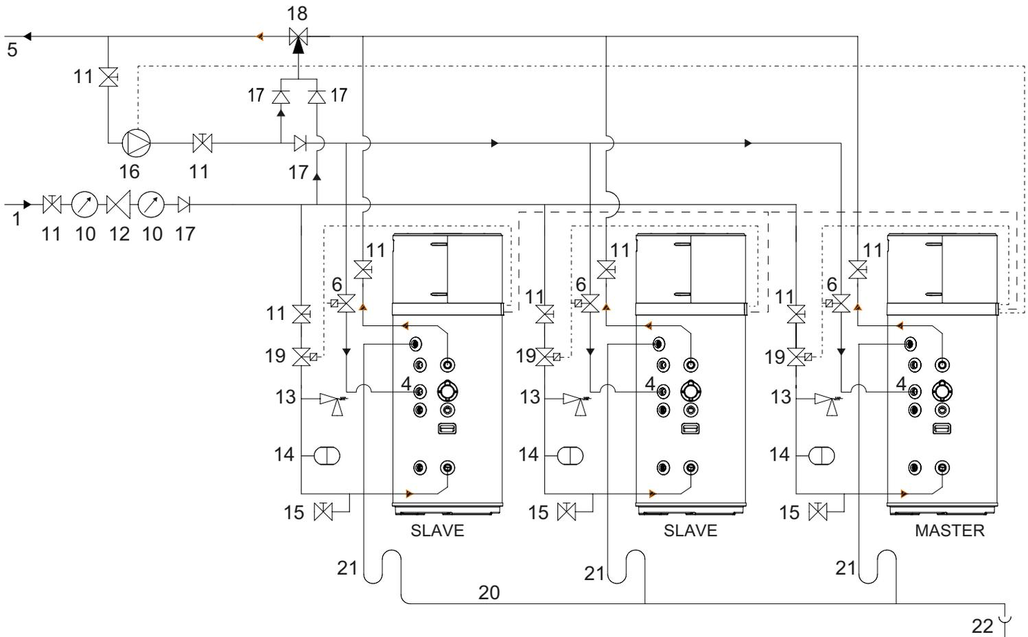
fig. 65 - Example of water system WITH thermostatic mixing valve (recirculation on unit water recirculation connection)
