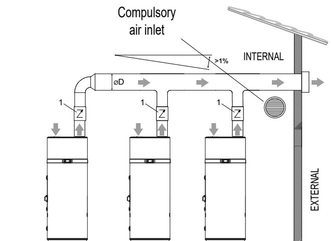
fig. 55 - Example of air discharge connection
